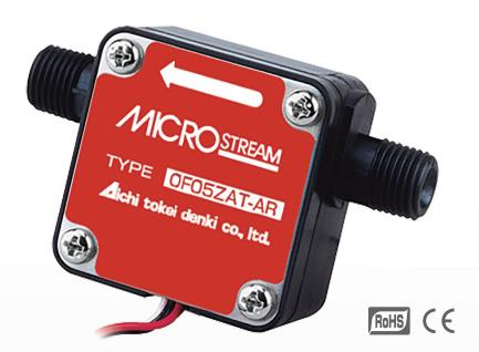
Microstream flowsensor OF-Z is ideal for measuring a variety of liquids and it is capable of measuring small flow accurately.
